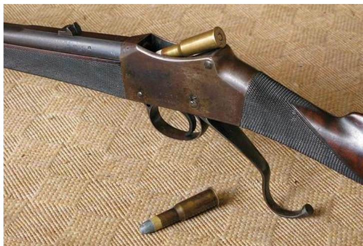
Martini Henry 450 rifle Weight 3.8 kgs; length 1.25m; calibre 12mm; range 1,700m
